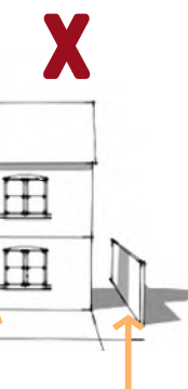
Extension too close to boundary with insufficient space for landscaping
