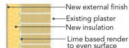
Externally insulated Stone Wall
