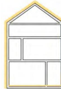
External Insulation Approach
