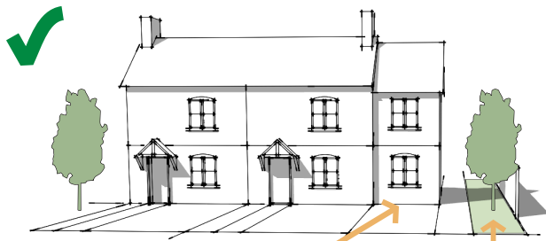
Subordinate side extension. Proportions in keeping with main dwelling.
