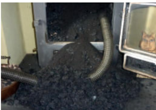
This stove is capable of burning very cleanly, the logs used were dry and the chimney was lined and insulated. But the owner got in to bad burning habits, closing the air controls off for long periods. The solid black "tar" or "creosote" nearly blocked this chimney. If there had been a chimney fire the liner would have been destroyed or worse. A lot of unnecessary air pollution was produced to create this much deposit in the chimney
